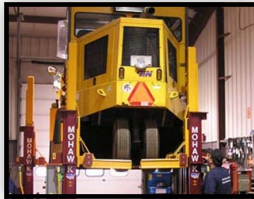
Street Sweepers Need 22" Lifting Forks
