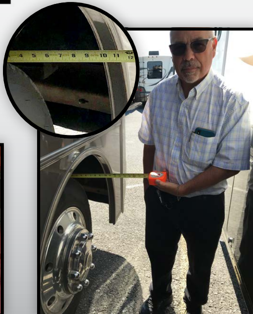
The inset of RV tires requires long lifting forks
